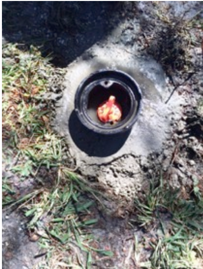
Monitor well with removable plug
