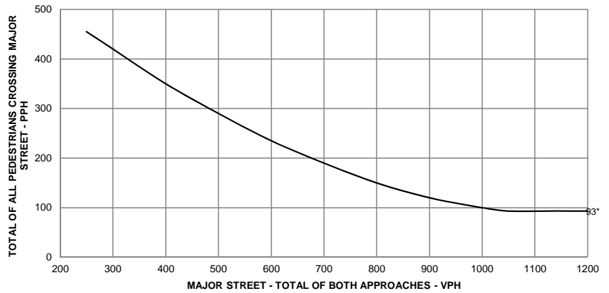
Figure 4C-8 Criteria for "70%" Volume Level - Peak Hour
