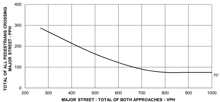
Figure 4C-6 Criteria for "70%" Volume Level
